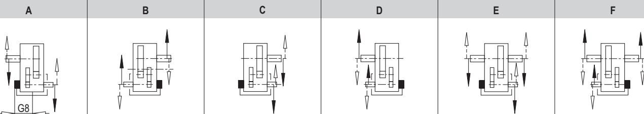
Dreistufig, Horizontal / Three stage, Horizontal - PH53-H ... 223-H / PH133-M ... 223-M
