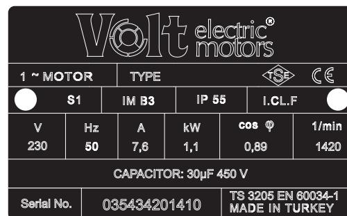
FIGURE 25: Single-phase motor nameplate
