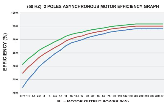
FIGURE 3: 2 poles Asynchronous motor efficiency power chart (50 Hz)
