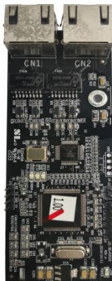
Ethernet/IP communication card EC-TX510/ EC-TX515
